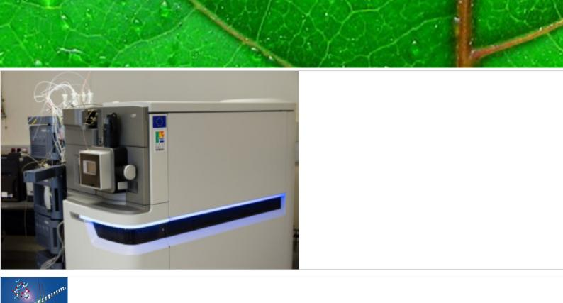
• A Gas chromatography – time of flight mass spectrometer
